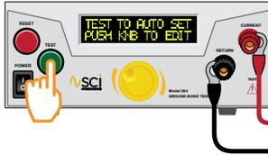
Push the green TEST button to start reading the offset value. CAUTION: The tester will start outputting once the TEST button is pressed.
