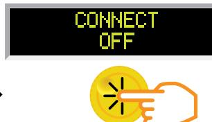
When **CONN** is selected. Press the rotary knob to edit the Connect Setting. The options will blink.
