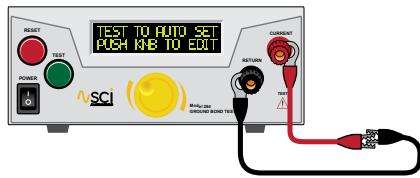
Short the Red High Current lead with the Black Return Lead as shown above.
