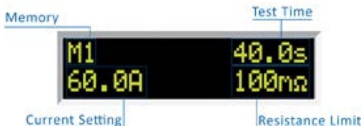
Follow the setup procedures to set the desired parameters. The display will show the Ground Bond test settings depending:
