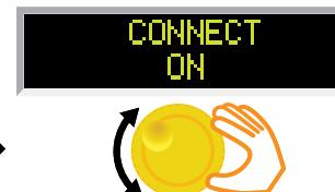
Turn the rotary knob to change the Connect setting: **ON** or **OFF**.
