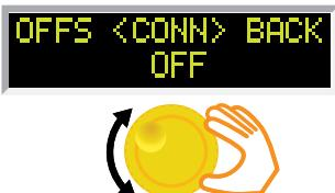
Turn the yellow rotary knob to scroll to desired parameter to edit **CONN**.
