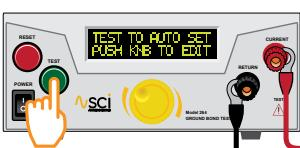
Push the green TEST button to start reading the offset value. CAUTION: The tester will start outputting once the TEST button is pressed.
