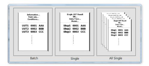
Batch - The Batch report contains all the test data displayed in the Unit Under Test (DUT/UUT) Result Table.
