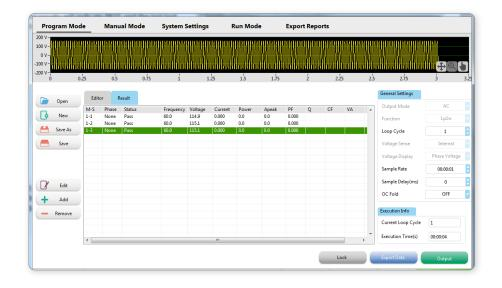
If a test sequence is aborted during the test, the step will be highlighted in red and the test status will be changed to Abort.
