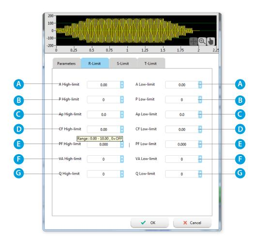
Moving the cursor over the parameter will display the available range for that test parameter.
