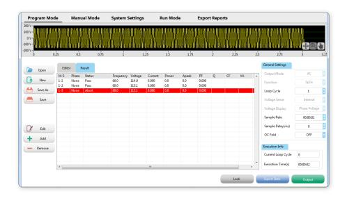
If the test sequence has any failed steps, the step will be highlighted Red. The test's status will change to the failure message reported by the power source.
