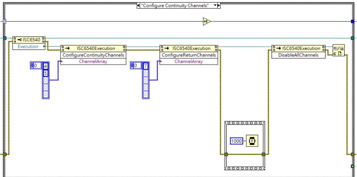
The **ConfigureContinuityChannels()** method takes an integer array as input. For the connection on the return circuits, we could invoke the method of **ConfigureReturnChannels()** which is shared with the withstand channels.
