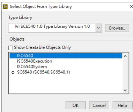
The Labview will automatically generate an **Automation refnum** of **SC6540Lib.ISC6540** control and connect to the Automation Open function.
