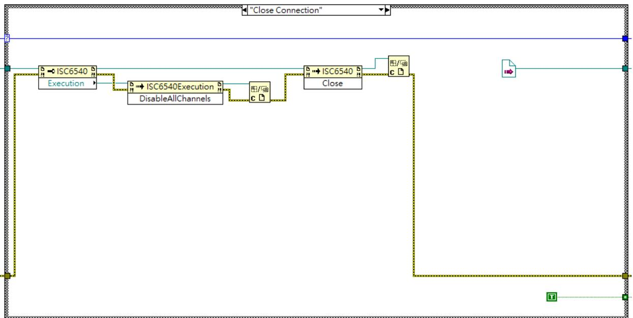
***Close()*** method in ***ISC6540*** class would close the I/O session to the instrument. Also, all of the references should be closed using the ***Close Reference*** function.
