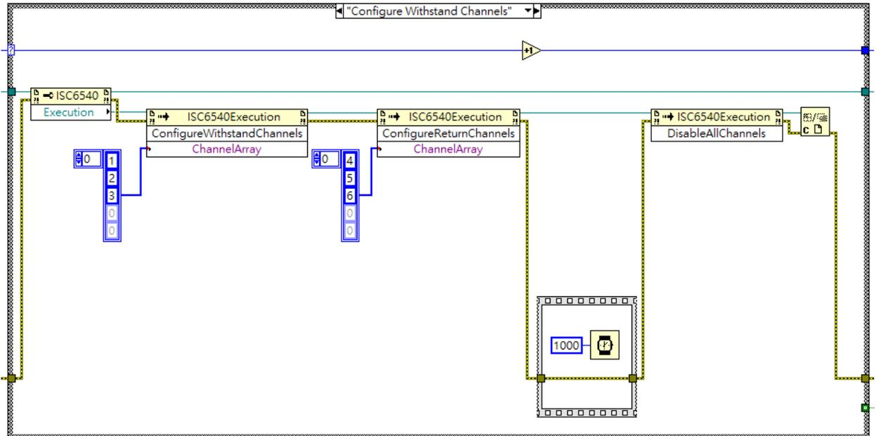
For some units, we may need a multiplexer, SC6540, to extend the capacity on a HIPOT tester, such as Omnia2, HypotUltra, Hypot4 of Associated Research. Before a withstand test operated, the multiplexer needs to be configured to the test point.
