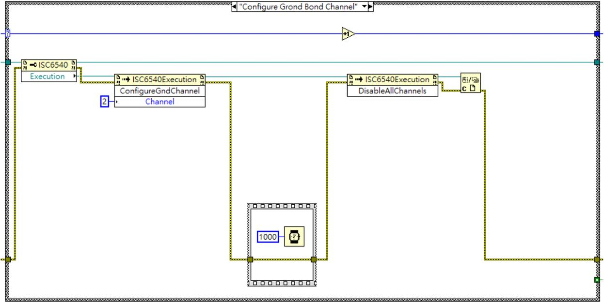
Only one ground bond channel could be enabled at one time. Therefore, the **ConfigureGndChannel()** takes a integer as input parameter at once. When a ground bond channel was set, the other switches would be disabled automatically.
