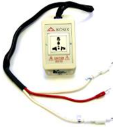
Figure 8: Universal Receptacle Box
