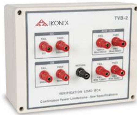
Figure 7: Associated Research TVB-2 Test Verification Box
