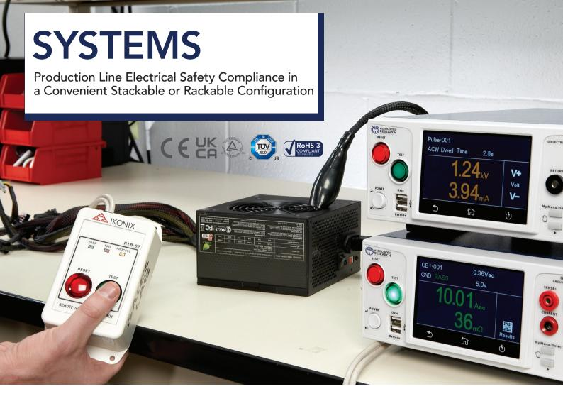
Interconnect our Hypot® Series Hipot Instrument with our HYAMP® Series Ground Bond instrument to form a complete safety compliance system. Easily operate both instruments from a single point of control on the production line or in a rack. All test systems are safety agency listed, include interconnect cables, and detailed directions on effortlessly interconnecting your system.
