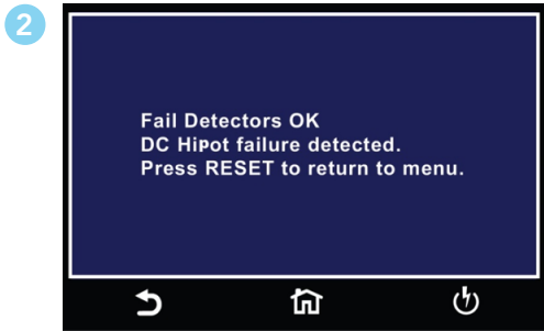
DC Hipot Fail Detectors OK screen.
