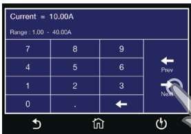
EDIT PARAMETERS Tap parameter values to edit individually. After you adjust each parameter, tap ENTER (↵) arrow key to save changes.
